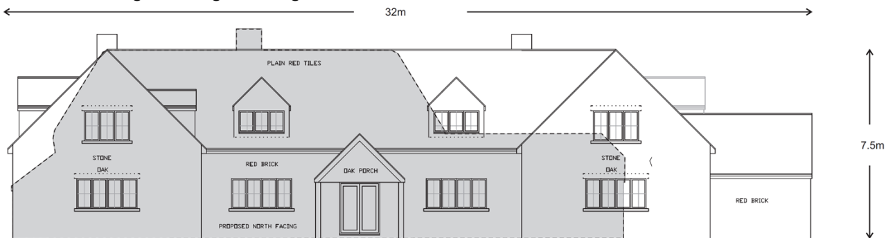
Proposed front elevation with the size of the previous cottage superimposed in grey for comparison
